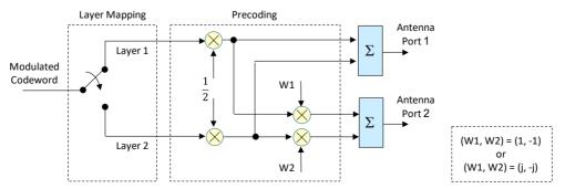
Figure 393 - Dual layer precoding applicable when CSI Reference Signal uses antenna ports 3000 and 3001
